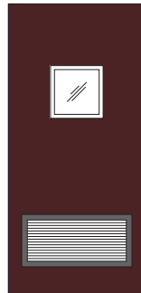
VS/BL – Vision square with Bottom Louver
